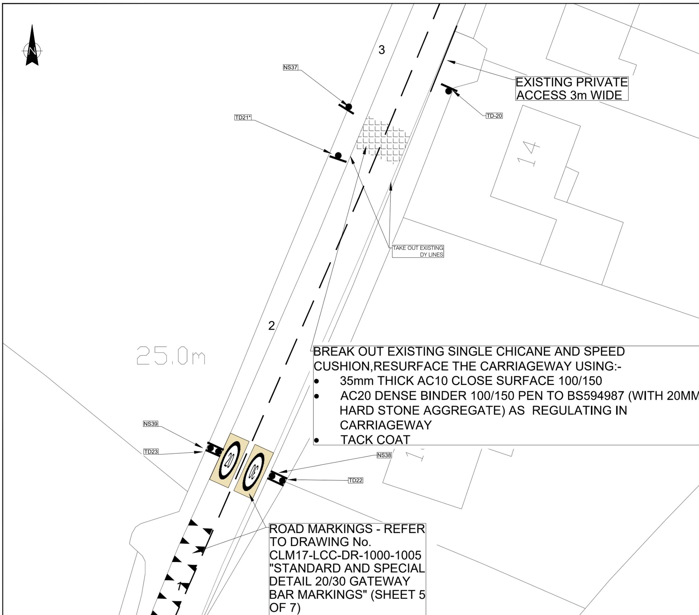
**BREAK OUT EXISTING SINGLE CHICANE AND SPEED CUSHION, RESURFACE THE CARRIAGEWAY USING:-**
